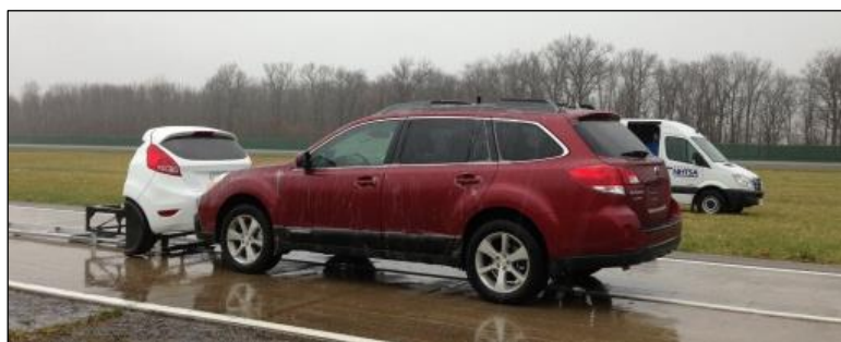
Figure 3-11. Subaru Outback CIB test performed in moderate rain
