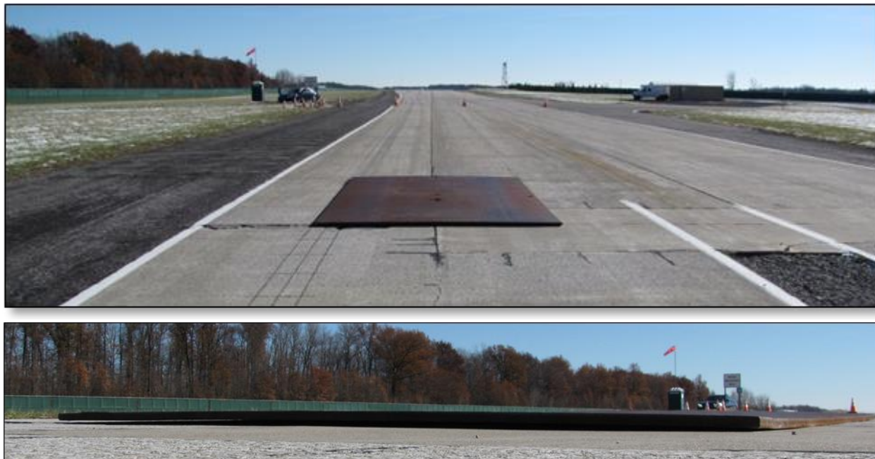
Figure 3-5. Steel plate used to evaluate unintended CIB/DBS activations
